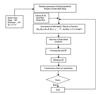
Figure 2: The flowchart of the genetic algorithm
