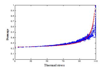
**Figure 7:** The influence of thermal stress on the interface damage ( $\sigma$  = 115 N/m<sup>2</sup>)
