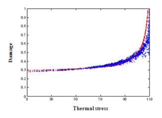
Figure 3: The influence of the thermal stress on the interface damage ( $\sigma$  = 105 N/m<sup>2</sup>)
