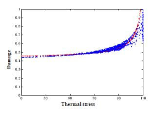
Figure 5: The influence of the thermal stress on the interface damage ( $\sigma$  = 125 N/m<sup>2</sup>)
