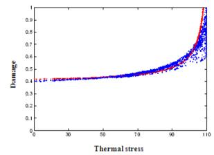
**Figure 4:** The influence of thermal stress on the interface damage ( $\sigma$  = 115 N/m<sup>2</sup>)
