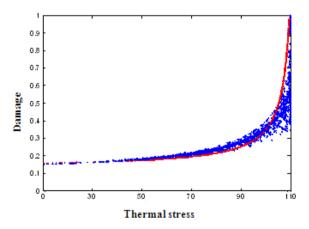
Figure 6: The influence of thermal stress on the interface damage ( $\sigma$  = 105 N/m<sup>2</sup>)
