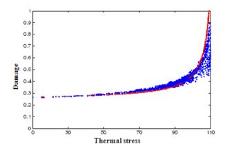
**Figure 8:** The influence of thermal stress on the interface damage ( $\sigma$  = 125 N/m<sup>2</sup>)
